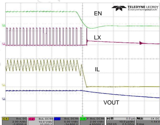
开关波形( $V_{IN}=12V, V_{OUT}=3.3V, I_{OUT}=0.1A$ )
