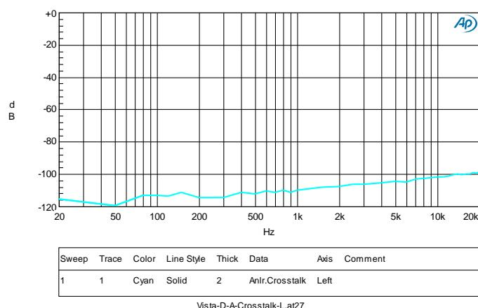
FIGURE 5. 48K/16BIT, 10K LOADING DAC, CROSSTALK R
