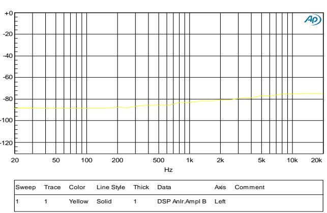
FIGURE 16. 48K/16BIT, MICROPHONE IN, CHANNEL SEPARATION R
