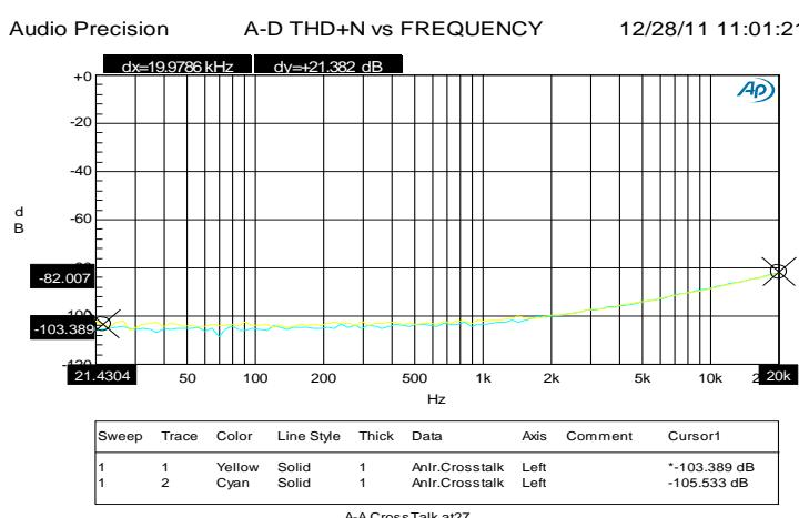
**FIGURE 35. LINE IN TO LINE OUT, CROSSTALK R**
