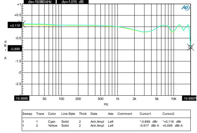
FIGURE 2. 48K/16BIT, 10K LOADING DAC, FREQUENCY RESPONSE
