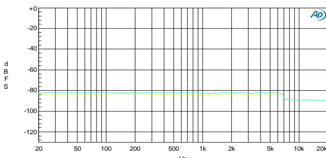
FIGURE 13. 48K/16BIT, MICROPHONE IN, THD+N
