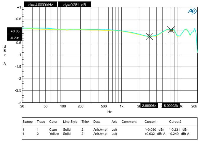
FIGURE 3. 48K/16BIT, 10K LOADING DAC, PASSBAND RIPPLE
