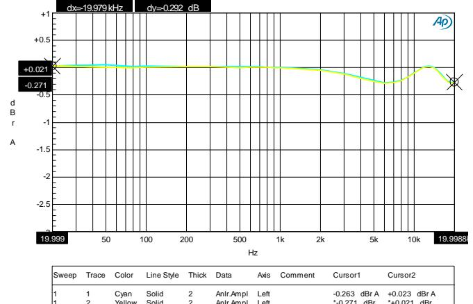
FIGURE 8. 96K/24BIT, 10K LOADING DAC, FREQUENCY RESPONSE
