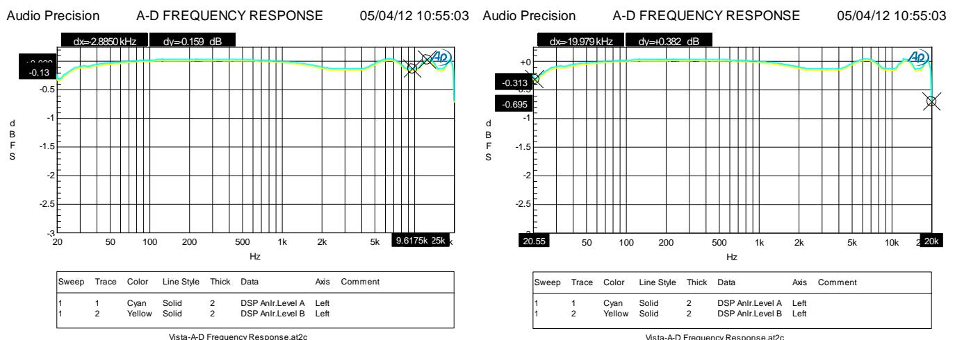
FIGURE 19. 48K/16BIT, LINE IN, PASSBAND RIPPLE
