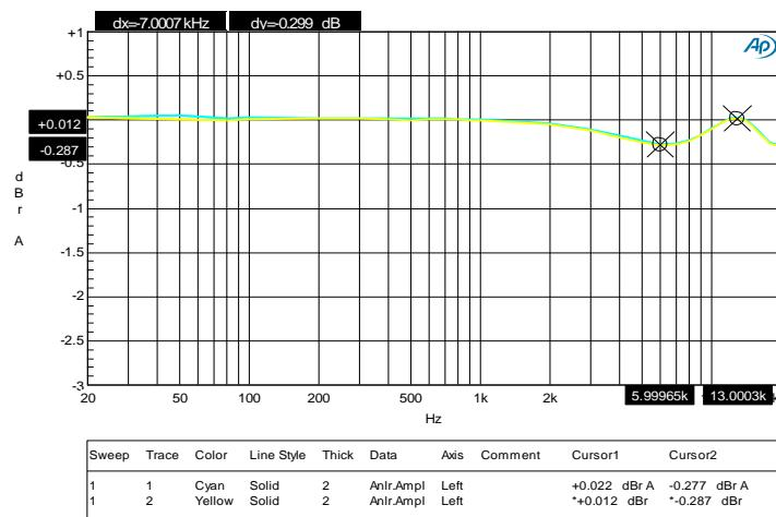
FIGURE 9. 96K/24BIT, 10K LOADING DAC, PASSBAND RIPPLE
