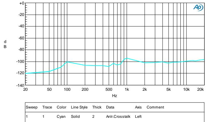
FIGURE 10. 96K/24BIT, 10K LOADING DAC, CROSSTALK L
