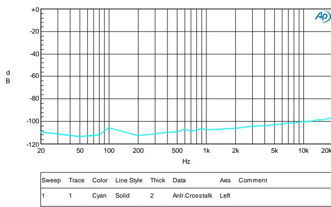
FIGURE 11. 96K/24BIT, 10K LOADING DAC, CROSSTALK R
