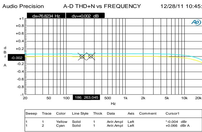
**FIGURE 33. LINE IN TO LINE OUT, PASSBAND RIPPLE**
