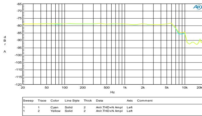
FIGURE 1. 48K/16BIT, 10K LOADING DAC, THD+N
