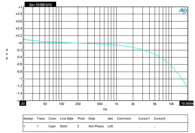
FIGURE 6. 48K/16BIT, 10K LOADING DAC, PHASE DELAY
