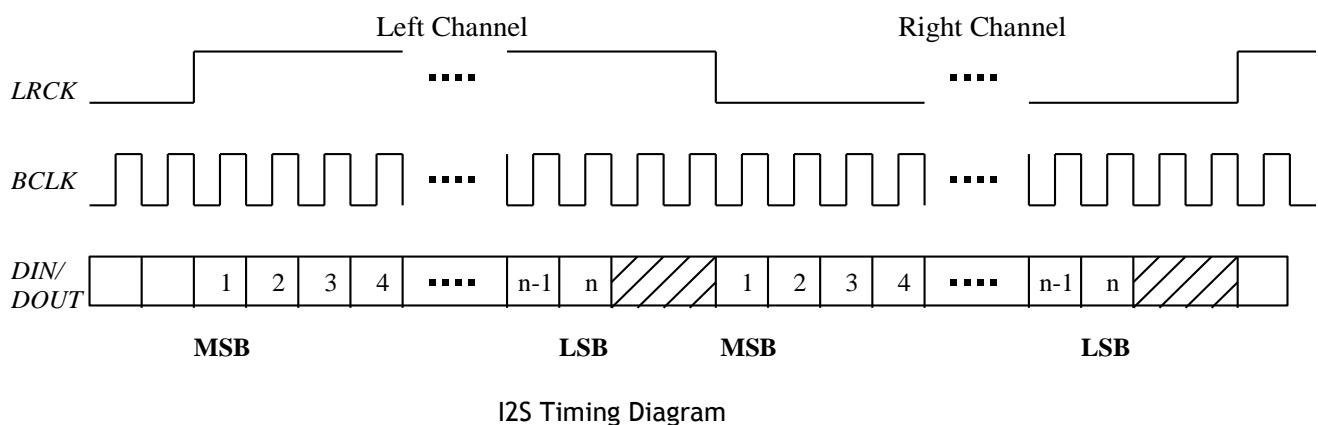
For the I<sup>2</sup>S DAC controller, the audio data is transformed from the parallel format to the serial format before transmission; then the bit data is shifted out one by one with the MSB first via DOUT signal. If the I<sup>2</sup>S DAC controller is set to 32 bits, at least 32 BCLKs must exist in both the LRCK left and right channels. In the same manner, the audio data is transformed from the coming serial format to the parallel format for an I<sup>2</sup>S ADC controller.
