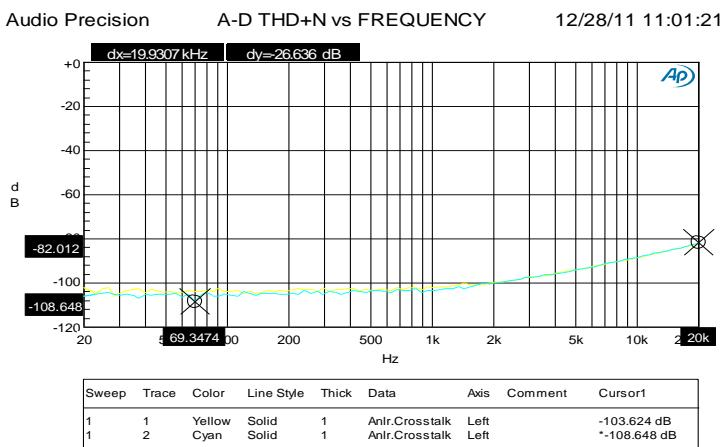
**FIGURE 34. LINE IN TO LINE OUT, CROSSTALK L**
