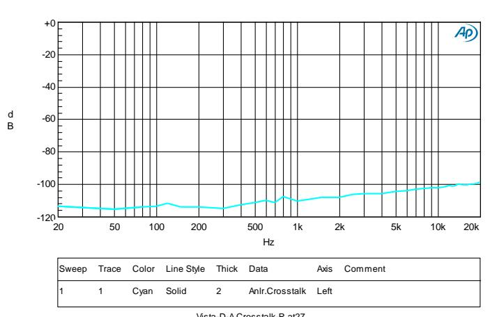
FIGURE 4. 48K/16BIT, 10K LOADING DAC, CROSSTALK L
